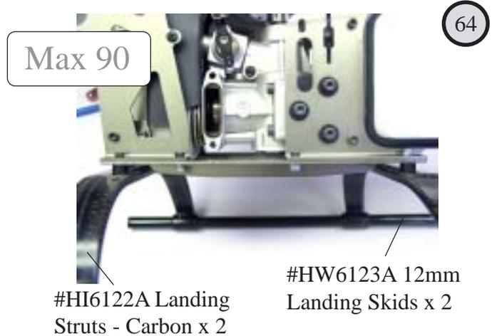
Attach the landing gear frame to the mechanics with M3x8 socket screws and locknuts. Attach the landing gear with M3x20 socket screws, M3x10 flat washers (against struts), M3x9x4 spacers and M3 locknuts, sliding the front skids into final position. Mark, scuff and bond the skids to the struts with JB Weld.
