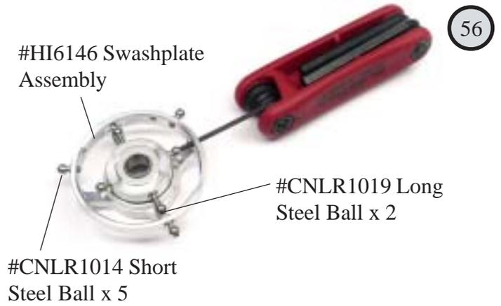
The double bearing swashplate requires no maintenance. If a steel ball needs changing, insert the 2.5 hex key through one of the extra holes in the outside ring. Two medium ball on the inside race.
