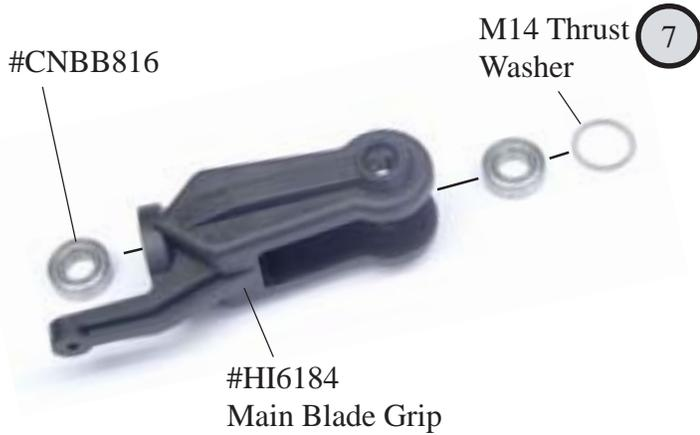
Insert one ball bearing into each end of the main blade grip. Slide the M14 Thrust Washer against the inside bearing.
