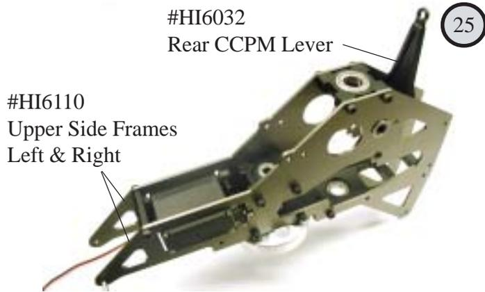
Install the rear ccpm lever into the upper frames flush with the bearing on the left side, having the mount extend out the right side frame. Assemble the upper frames but do not use locktight at this time.
