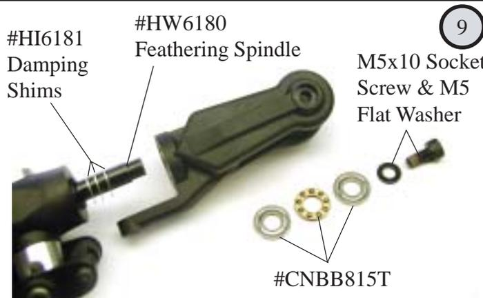
Slide three shims onto the feathering spindle, followed by the blade grip assembly. Pitch arm is on leading edge. Grease and install the thrust bearing and secure with the M5x10 socket screw and washer using threadlock.
