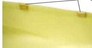
Bond the wood inside mounts into the inside of the canopy with Epoxy. Center each block over the holes with the top edge flush to the canopy edge. Once cured, drill the final hole size for the screws.
