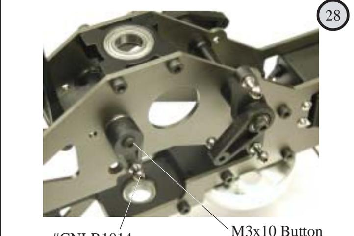
Press the rear ccpm lever onto the mount that sticks out of the right side of the upper frames with the steel ball downwards. Secure with the M3 button head screw.
