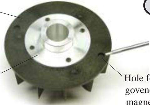
If a governor is planned to be installed, install the magnets into the holes already molded into the bottom of the cooling fan.
