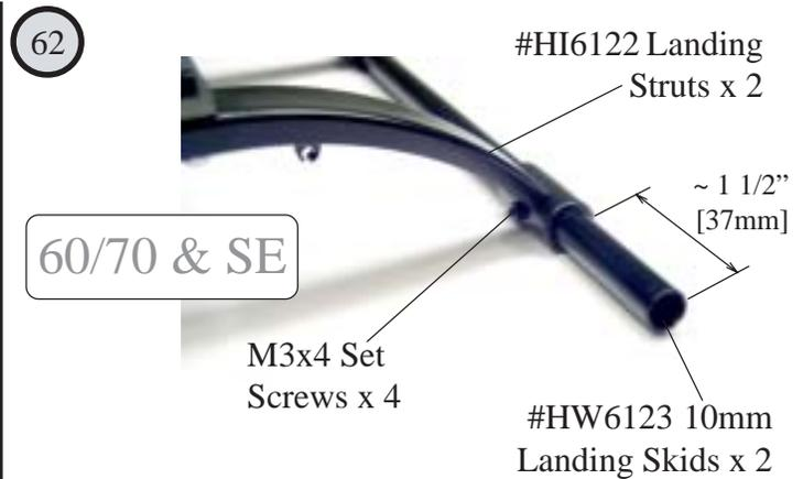
Assemble the landing skids onto the struts, note the correct direction is to have the struts sweep forward. Position the rear strut at approximately 37mm from the end and secure the skid with the M3 set screw. Leave the front loose for now.
