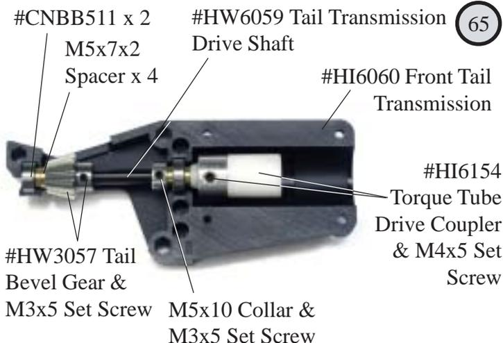
The front tail transmission is assembled. Open and apply locktight to the back edge of the bevel gear for added security.
