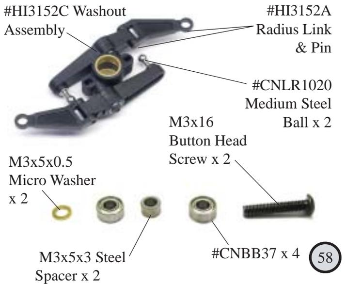
The washout unit comes assembled. Slide onto the main shaft and ensure that the screw is on the left side of the main shaft.
