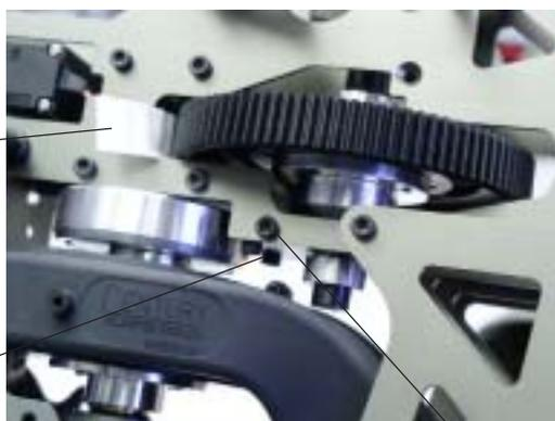
Remove and locktight M3x8 Socket screw.
