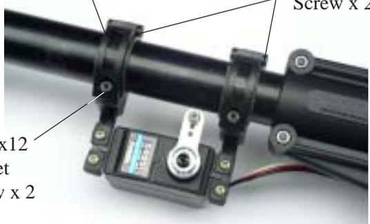
Wrap the tail mount liners around the tail boom and trim if necessary. Install the rudder servo mount assembly onto the tail boom, over the liners and secure using the M2.5 socket screws. Leave these loose until after the tail pushrod has been attached. Attach the rudder servo horn, positioning the steel ball at 12-14mm from the servo center.
